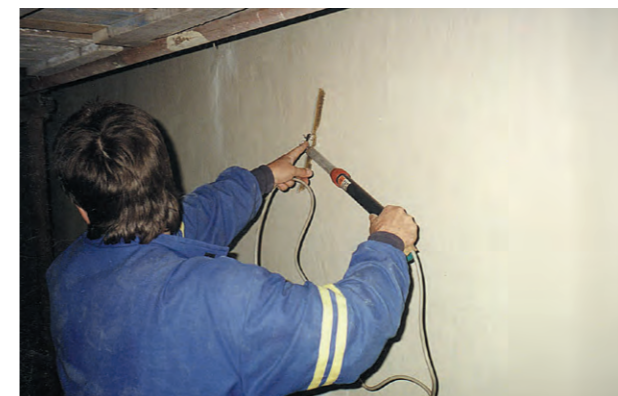
Kontrola celistvosti jiskrovou zkouškou Control of the integrity via spark test
